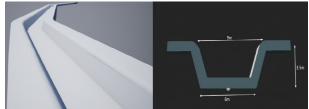
Fig. 5. The dimension and shape of the canal structure before adding any feature
