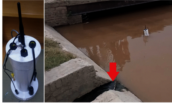
Figure 1-1: Mobile water quality monitoring sensor developed at Center for Water Informatics (WIT) [15]
