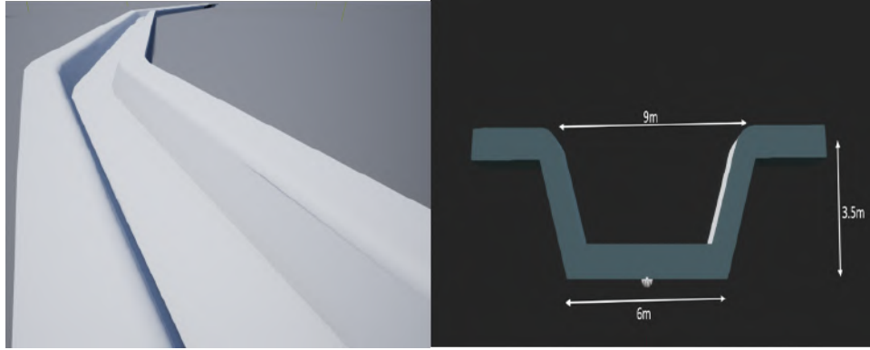
Figure 3-5: Canal 3D mesh, build in Auto Desk and then imported into Unreal engine.
